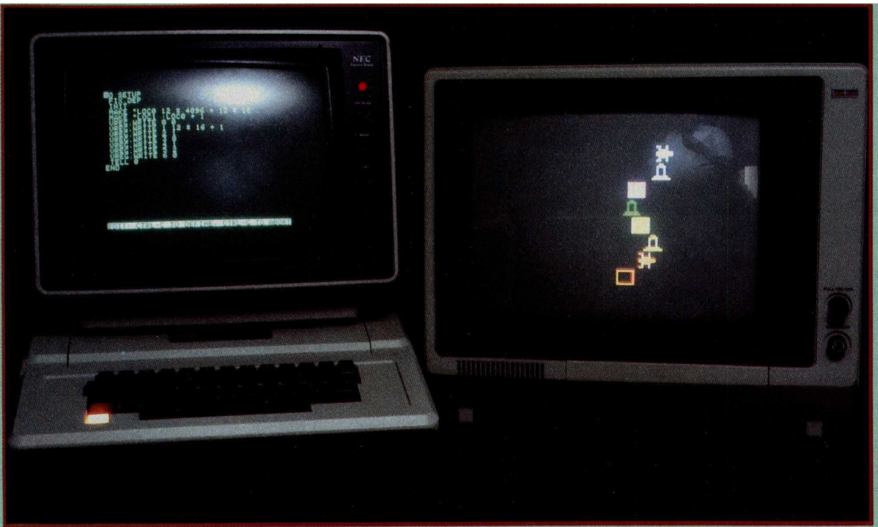
Photo 7: When the E-Z Color Graphics Interface is installed in the Apple II, the regular display screen is still used for Terapin MIT Logo's text display and turtle graphics; the E-Z Color board must be connected to a second color video monitor for its display to be simultaneously visible.
